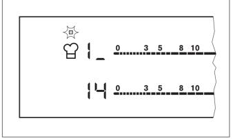
Heat setting display for the left front control bar shows the heat setting. To change the heat setting use left front control bar.
