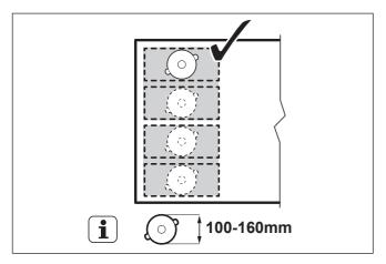
Place any cookware with bottom diameter larger than 160 mm centrally between two sections.
