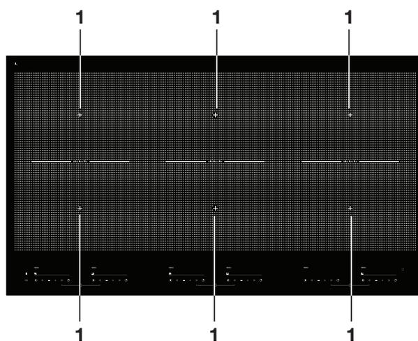
1. Adaptive zone 180 x 220 mm 3,7kW (zones that can be connected)
