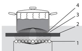
*The coil (1) in the hob (2) generates a magnetic field (3). By placing a pan with an iron base (4) on the coil, a current is induced in the base of the pan.*
